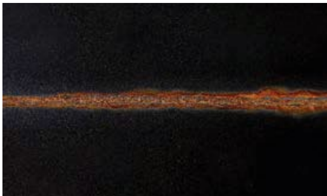
Figure 2. Three-layer standard coating system: 2-pack zinc dust epoxy-primer, DFT: 80 \mu\text{m} + 2-pack epoxy-intermediate layer, DFT: 120 \mu\text{m} + 2-pack polyurethane top coat, DFT: 80 \mu\text{m}
